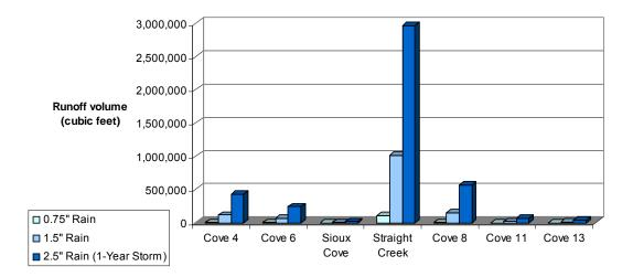
Figure 6. Volume of stormwater runoff entering Lake Waynoka tributaries during 0.75-inch, 1.5-inch and 2.5-inch storm events (NOTE: A 0.75-inch storm is used for water quality calculations by the EPA and a 2.5 inch storm event is considered a storm that has a 99% chance of happening every year)
