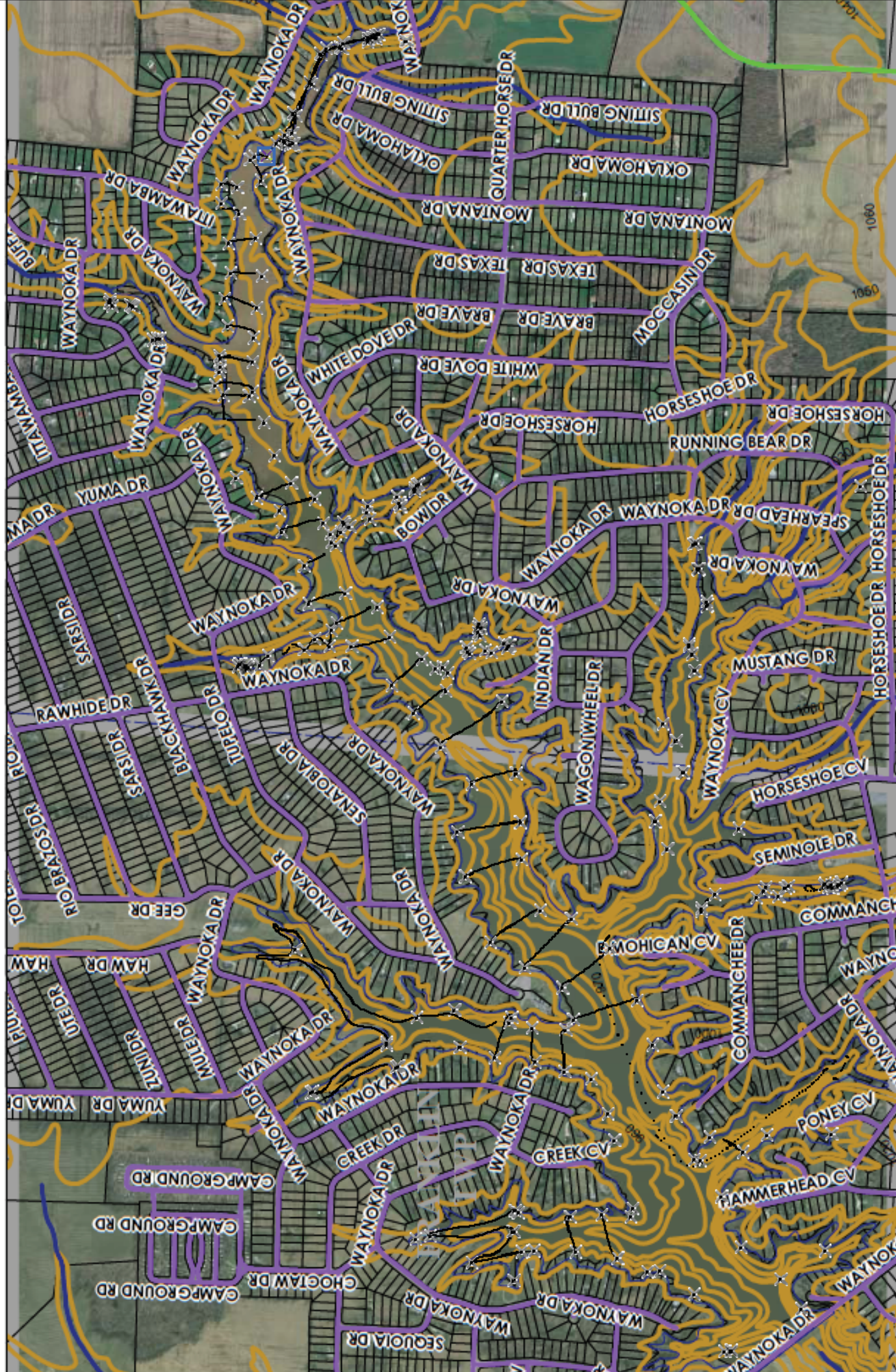
Figure 1. The locations of each transect traveled by the RiverSurveyor is shown on this aerial which is overlain with the 1961 topographic map. The black lines indicate the transect and x's indicate the starting and stopping locations. This aerial with the topographic overlay can be obtained from the Brown County GIS website.
